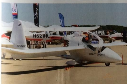
Ekolot Elf single-seat, all-composite motorglider.
